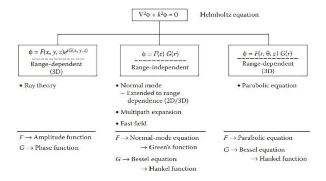
**Figure 1.** Summary of relationships among theoretical approaches for propagation modeling. (Adapted from Jensen, F.B. and Krol, H. 1975. The use of the parabolic equation method in sound propagation modelling. SACLANT ASW Res. Ctr, Memo. SM-72.)
